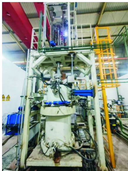
图 10 成都先进金属材料产业技术研究院 50 kg 加压电渣炉 Fig. 10 The equipment of 50 kg PESR furnace in Chengdu Advanced Metal Materials Industry Technology Research Institute Co., Ltd.
